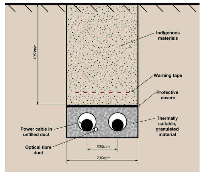
Typical Underground HVDC Arrangement
